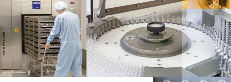
Manual loading of ampoules into a sterilizer
